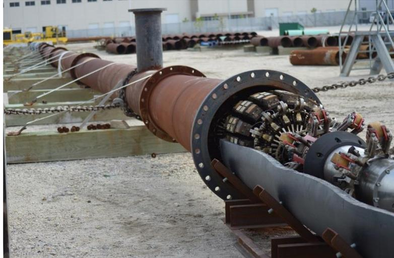
Figure 10 Launch of 24" EMAT ILI at the PRCI Pull Test Facility
