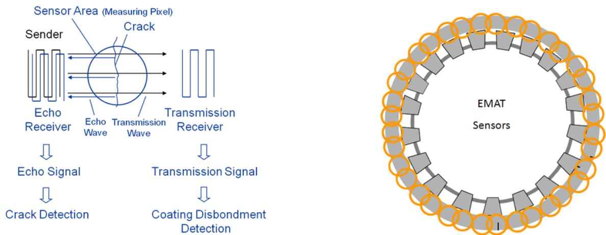
Figure 3: EMAT measurement principle and high resolution approach used by the Rosen EMAT-C ILI tools
