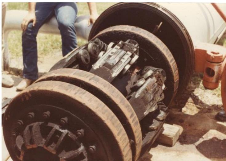
Figure 1: First ILI EMAT prototype developed by AGA and Rockwell in 1972
