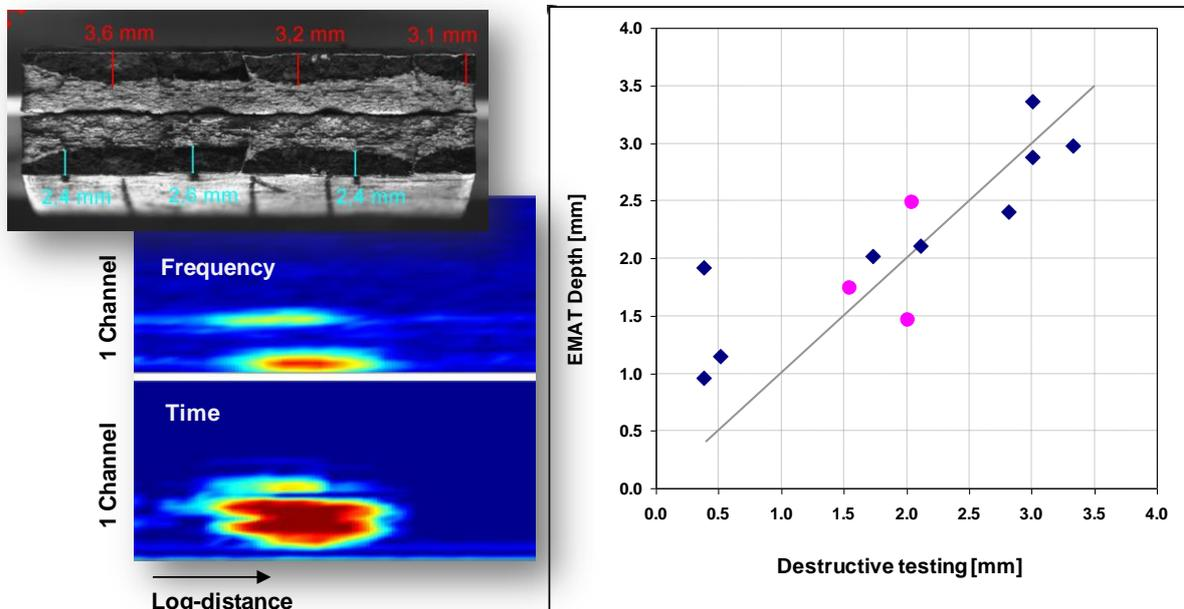
Figure 4: Depth sizing accuracy validated through destructive testing (splitting) of SCC.
