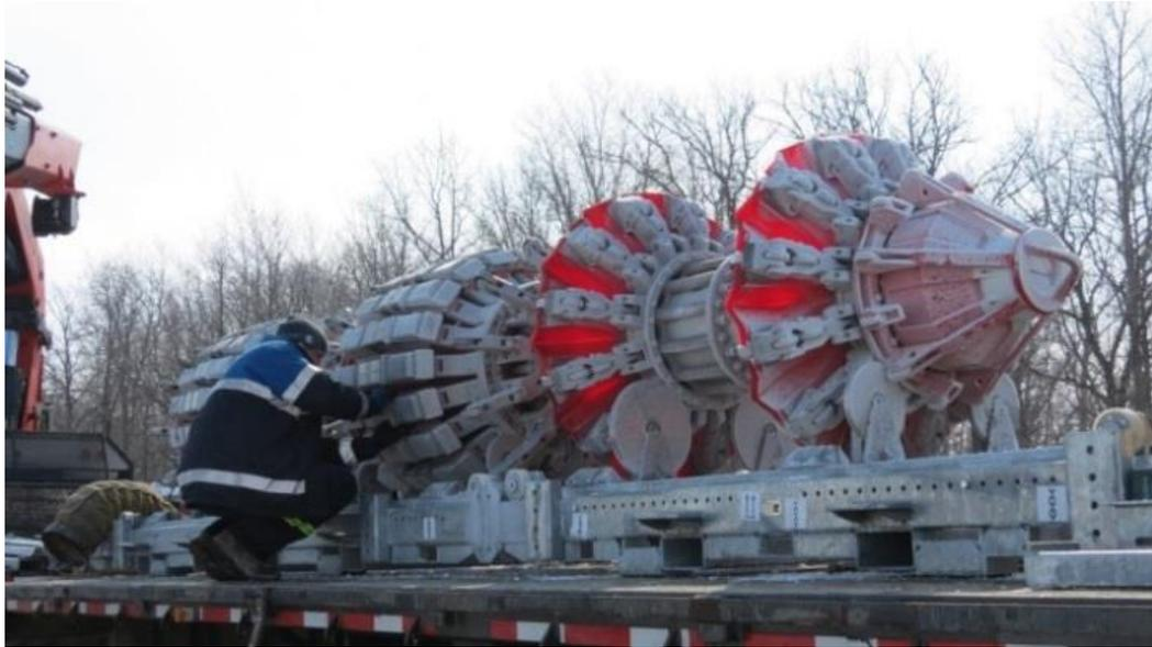
Figure 2: State of the art EMAT ILI tool for the detection of axial cracking in gas pipelines. On the right the pull unit with central suspension and wheel support is visible. On the left the two EMAT measurement units are shown.
