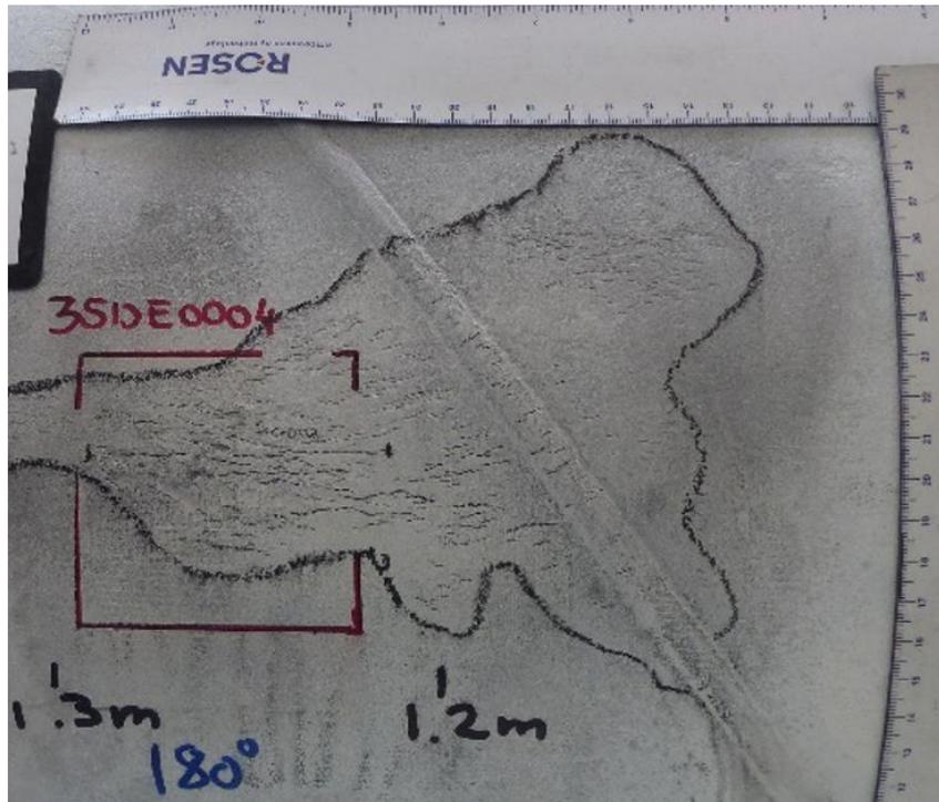
Figure 6: Corrosion and Cracking at the same location
