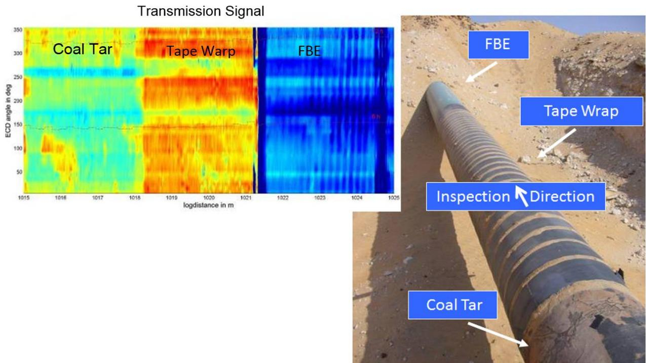
Figure 5: Different coating types and their characteristic transmission signal patterns in the EMAT data
