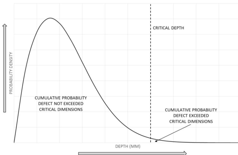
Figure 3: Probability of exceedance for defects (cracks) depth
