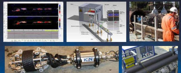
Self propelled BiDi Tethered Inspection Tool Technology
