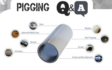
Figure 2. Geohazards can change the shape of a pipeline and may create local features, such as dents, buckles, ovalities and bending, all with potentially detrimental effects on the pipeline's integrity.
