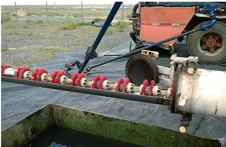
**Subtitle:** ROSENs new 4 inch combined inspection tool at the launcher trap in Kazakhstan.
