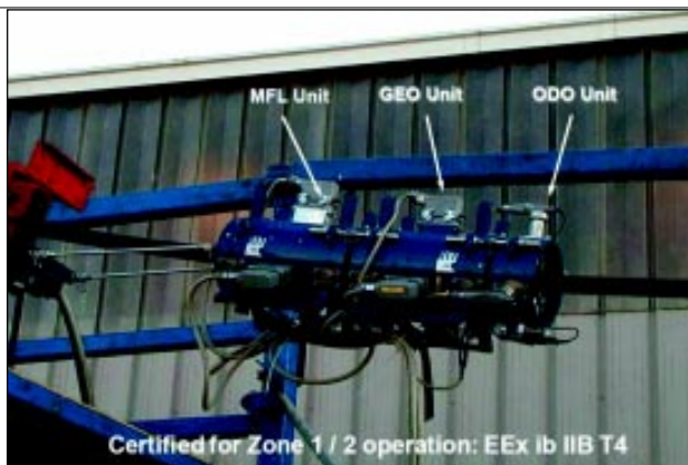
Figure 5: Mfl unit, Geo unit, Odo unit, MFL sensor cable and Geo-Odo sensor cable
