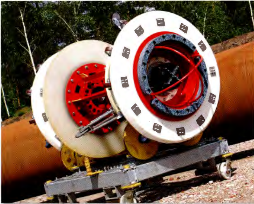
Fig. 2. ROSEN's acoustic leak detection tool.
