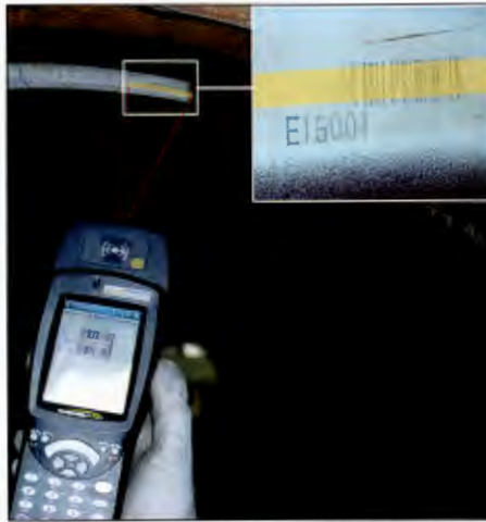
Fig. 8 Transmission of pipe number from barcode to RFID chip
