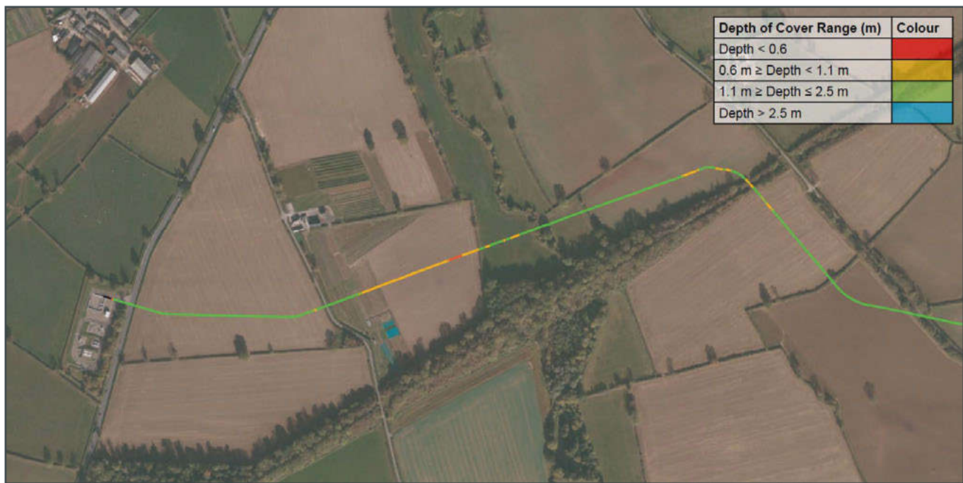
Figure 2: Example Depth of Cover Report (Aerial imagery source: Esri, DigitalGlobe, GeoEye, Earthstar Geographisc, CNES/Airbus DS, USDA, USGS, AeroGRID, IGN and the GIS User Community)
