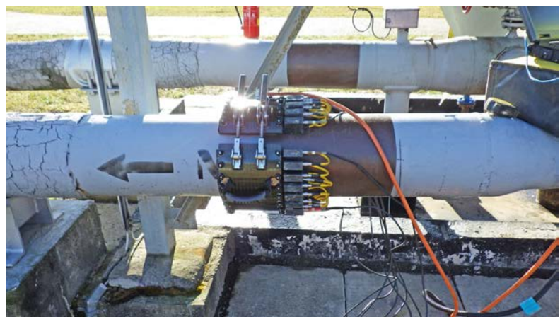
Figure 5. LRUT collar with multi-mode modules and transducers sending soundwaves for tens of meters in both directions.
