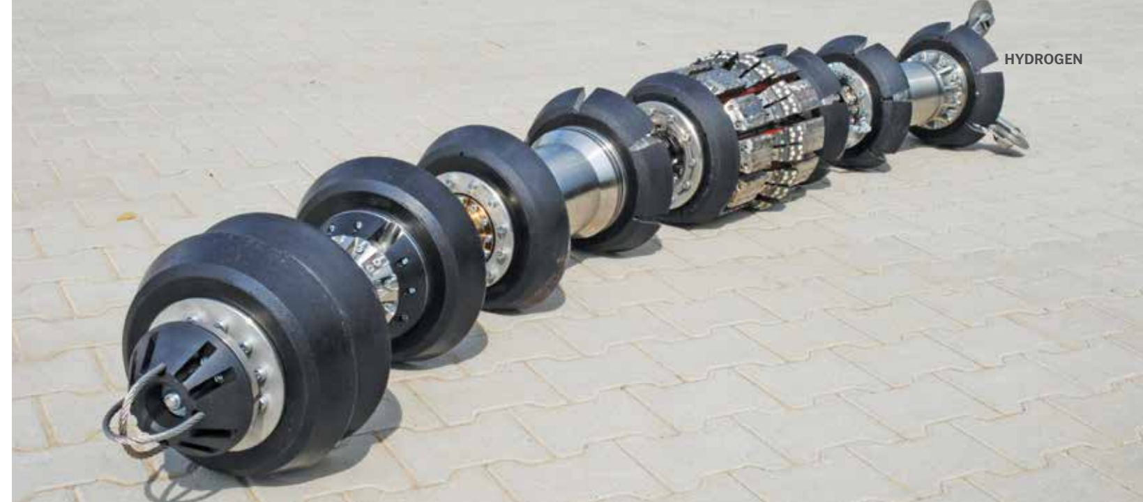
The ATEX-compliant MFL ILLI tool.
