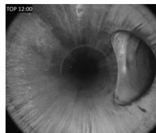
Figure 4: Verification of an unbarred tee
