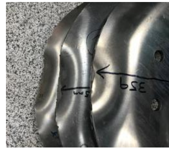
Figure 2: Gauge plates with unexplainable deformation
